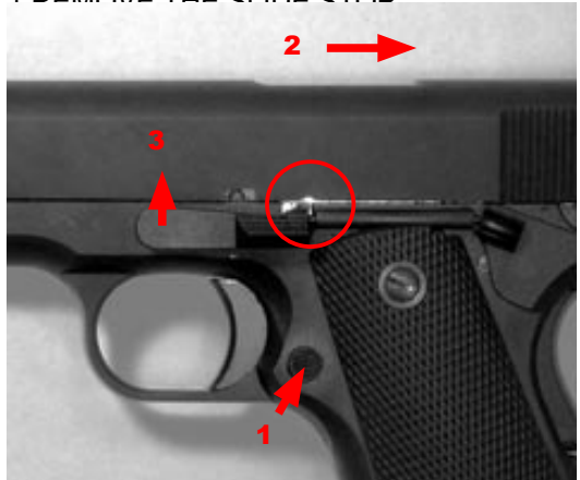
THE SLIDE REAR UNTIL THE TAKEDOWN NOTCH IS JUST ABOVE THE SLIDE STOP TAB AND REMOVE SLIDE STOP
