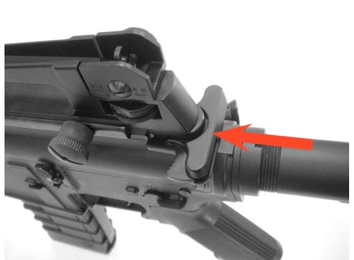
DEPRESS GUARD PLUNGER AND OPEN THE TRIGGER GUARD WHEN WEARING ARCTIC MITTENS
