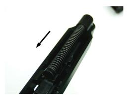
REMOVE THE RECOIL SPRING GUIDE AND SPRING.
