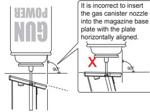
It is incorrect to insert the gas canister nozzle into the magazine base plate with the plate horizontally aligned.
