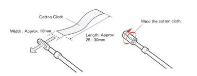
Cut a cotton cloth to the size shown above and insert one end into the hole in the rod. (Adjust the length of cloth for smooth entry into the barrel.)
