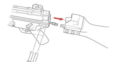
3 Loosen the screw on the rear of the gearbox, take off the pin, then pull out the lower receiver.
