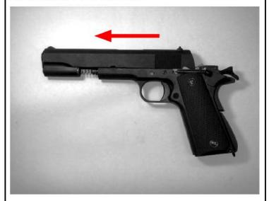
3.REMOVE THE RECOIL SPRING AND SPRING CAP
