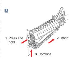
依順序壓下固定環再將護木接上。 Press and hold the delta ring. Insert the handquard back to place.
