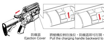
Pull the charging handle backward to open the ejection cover for hop-up adjustment.
