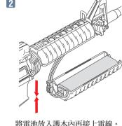
將電池放入護木內再接上電線。 Place the battery inside the handguard and then connect the connectors.
