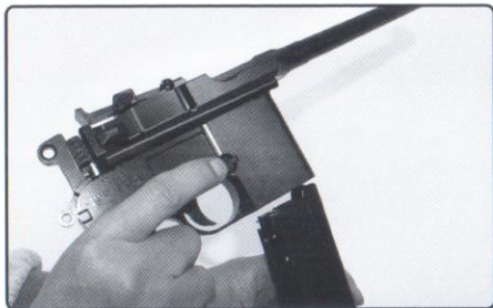
按下退彈匣鈕 Press in on the magazine catch and remove the magazine.
