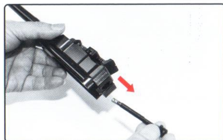
取出覆進簧桿 Remove the recoil spring guide rod.
