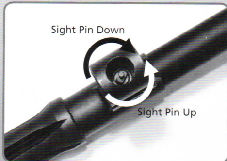
You can using pliers to adjust the Front Sight Pin.
