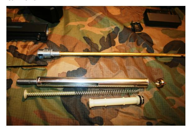
The hopup chamber is made out of metal and seems to do its job. The hopup rubber though is made out of low quality rubber. Unfortunatly without modification you can not put standard AEG or VSR type hopup rubbers into this rifle. The only other upgrade hopup replacement is the PDI Type 96 hopup chamber.
