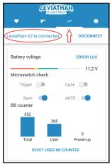
5. Check if every micro switch responding. They are displayed on picture 6 and 7. Grey color is OFF, blue is ON. There is delay about 1s because of BT communication. Move sector gear slowly to show "Cycle, detection. With selector on auto are semi and auto detection ON (like on the picture).
