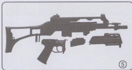
上下机匣分解完成 Upper and down casing is finished disassembling
