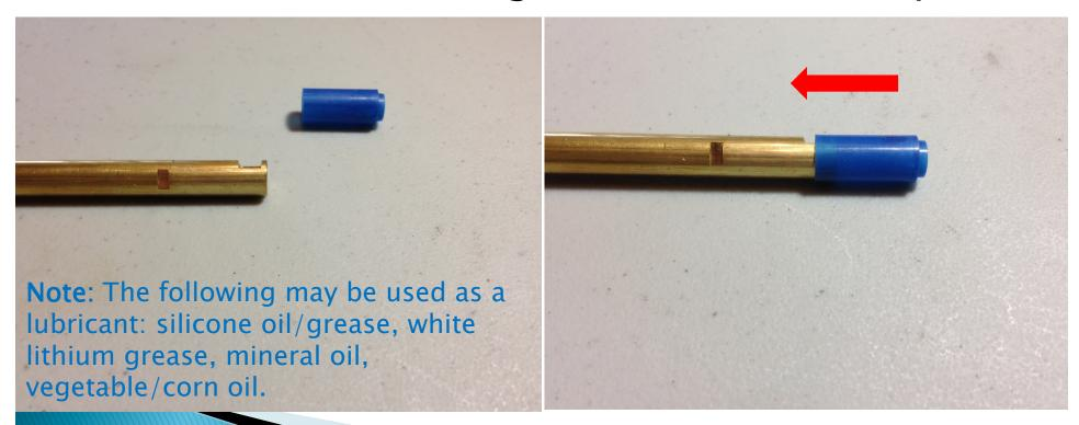
Care must be used when seating the internal contact patch of the bucking inside of the barrel window. Use your index finger and thumb to pinch the sides of the bucking and push upward and then over to clear the breach ring on the barrel. This will prevent damaging the internal contact patch of the bucking during installation.
