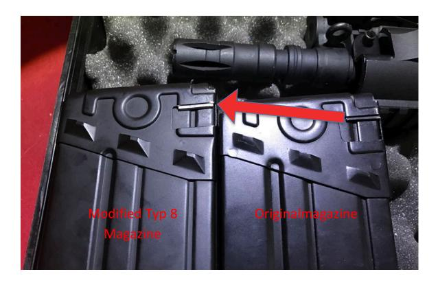
To solve the problem, a small piece of metal/plastic (for instance of an old magazine case, PC housing, storage boxes, CD) must be stuck in the mag catch window of the magazine. With hit piece installed, the magazine is pushed further into the magazine well and the feeding problem disappears.
