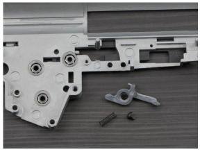
1.5 Clean the gearbox case using solvent.
