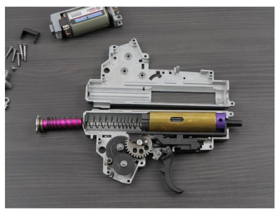
1.4 Disassemble all the internal parts (cylinder set, spring with spring guide, gears with anti-reversal latch, trigger, trigger switch, cut-off lever with spring).
