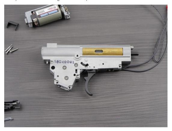
5.3 In some replicas (G36, UMP, etc.) you need to modify the mechanical trigger lock, because it is too long and touches the TITAN's top board. In this case, grind the protruding element by around 1.5/2mm.
