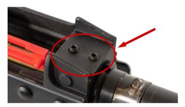
Once you have loosened the marked screws, the outer barrel can be pulled out of the housing towards the front. The original HopUp Unit together with the inner barrel can now be removed from the housing at an angle and dismantled.
