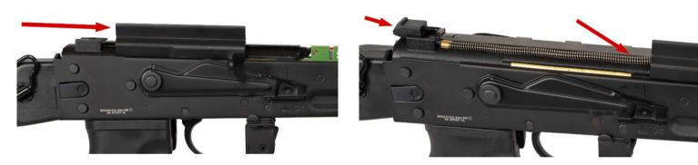
Your new HopUp system is now successfully installed. You can now increase or decrease the hop-up effect using the adjustment wheel. If a new HopUp rubber was installed, it should be shot in with 200 - 300 shots.
