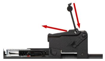
If you have loosened the marked screw, the outer is only held by the lateral bolts. Tap it out and pull the outer barrel forward out of the case. **Attention: Not every manufacturer uses a bolt here!** If this is not the case with your weapon, the outer barrel is only held in place by the inner screws.
