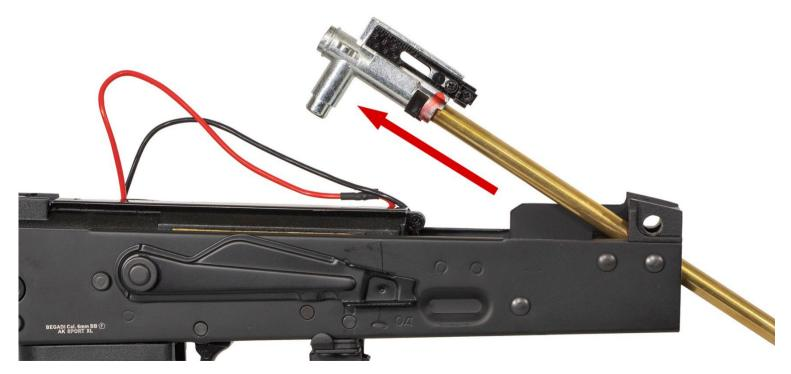
If you want to keep the original inner barrel, remove the front plastic clip downwards. The barrel can now be pulled out of the unit.
